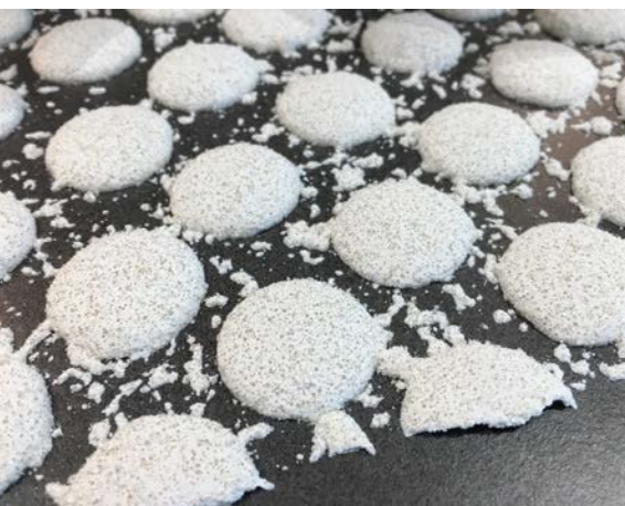
Reflective glass beads in a multi-dot structured road marking
