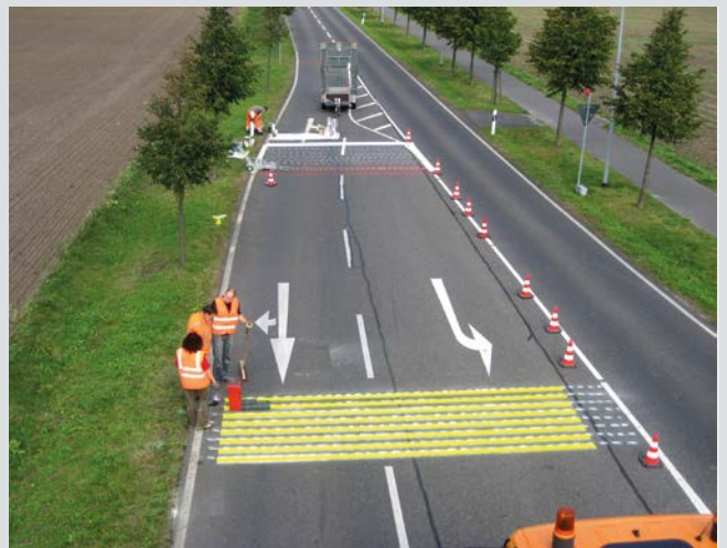
Always working very closely with the product: The laboratory and field testing staff Heidi Ehlert, Frank Siegmund and Patrick Wesche from SWARCO Limburger Lackfabrik evaluate the latest rumble strips for traffic calming purposes.
